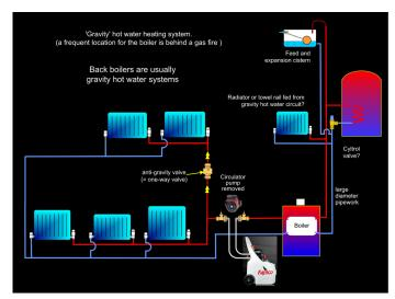
However, this will not clean the gravity hot water pipework. Some engineers will re-locate the Clearflow pump and connect it across the cold feed and expansion piping to force water through the gravity hot water circuit.
