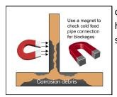
completely blocked you will have to cut the pipe work section out. Start cutting!
