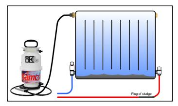
If you can't clear a radiator on a microbore system, it may be that a plug of sludge is blocking the narrow diameter pipework leading back to the manifold. If you have a Kamco Systemsure IK6 injector, the following can be worth trying to restore flow to the radiator.
