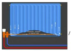
water towards the far side of the radiator) has broken away, so that the entrance and exit are effectively only 15-20mm apart, any flushing effect on that radiator will be minimal. Conversion to opposing inlet and outlet valves is a better long term proposition.
