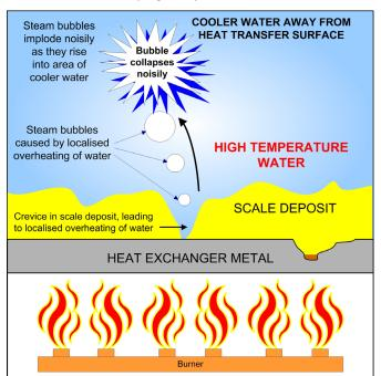
surface. This means that the metal runs hotter than design temperature and may even exceed 100 degrees C. The layer of scale / debris is never even, and there will
