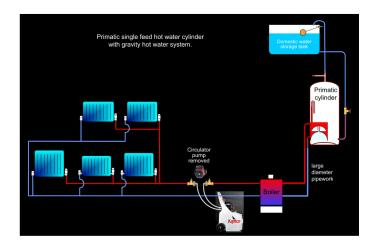
This would have to be power flushed separately, ideally by connecting across the system circulator pump connections.
