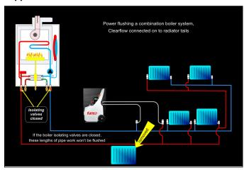
A. You'll need to flush this separately with a hose pipe (so pick a small radiator!).
