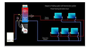
2. If you do include the thermal store in the power flushing circuit, then instead of pumping approximately 100 or less litres of water around, you'll be pumping around almost three times that, and so the vital overall flow rate will be much less than half – so not a good idea
