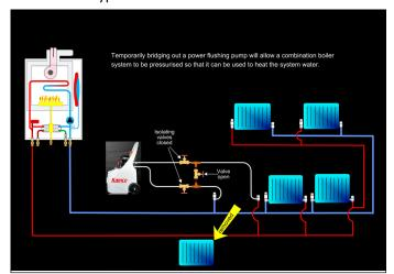
You now have a temporarily completely closed circuit, and so re-pressurise this the normal way, and then fire up the boiler until you have the system water good and hot. When you've got it up to temperature, shut off the boiler and use the valved manifold to put your power
