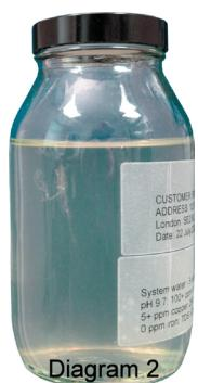
2. A clear sample of water does not eliminate the possibility that corrosion has taken place in the past and that there may be substantial corrosion debris present in the base of radiators and under floor sections, having settled out over time. This occurs because the circulation rate of a standard system circulator is not enough to keep debris in suspension.
