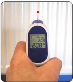
To use, aim the infrared thermometer at the target and press the trigger to measure the surface temperature. The word 'SCAN' will be shown at the bottom of the display. Release the trigger. The word 'HOLD' is displayed and the temperature reading is held for 10 seconds, after which time the thermometer will shut down. Note: Holding the trigger
