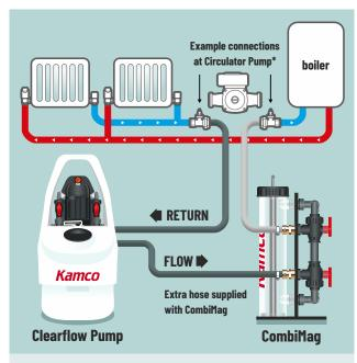
\*Flow and return may be connected at circulator pump connectors or using the **Kamco CP2 Pump Head Adapter**, or at many alternative points in the system.
