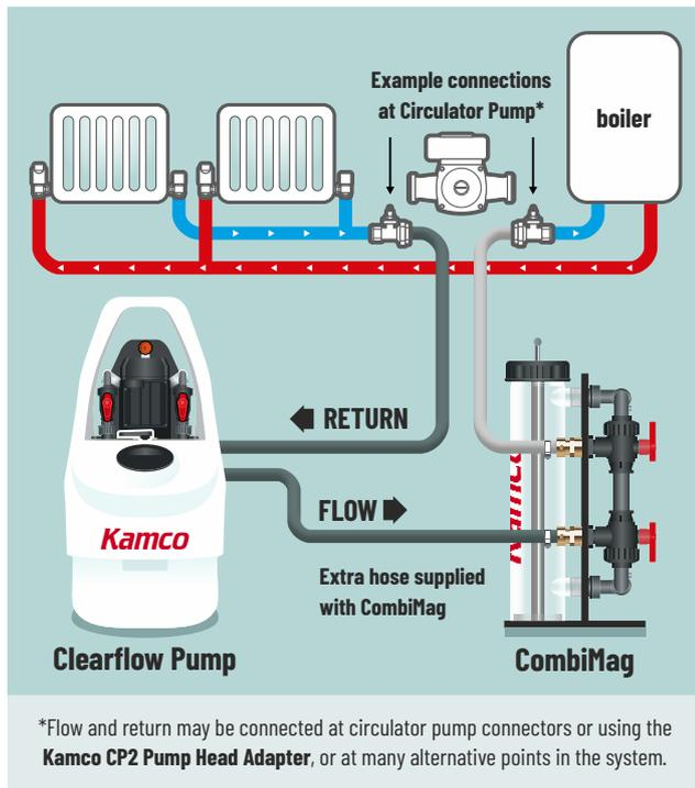
The power flushing pump can circulate the system water in either direction by operation of the flow reversing lever. However we suggest that the initial set-up is such that the **CombiMag** filter is installed before the boiler to offer the boiler a higher level of protection in the early stages of the power flush.
