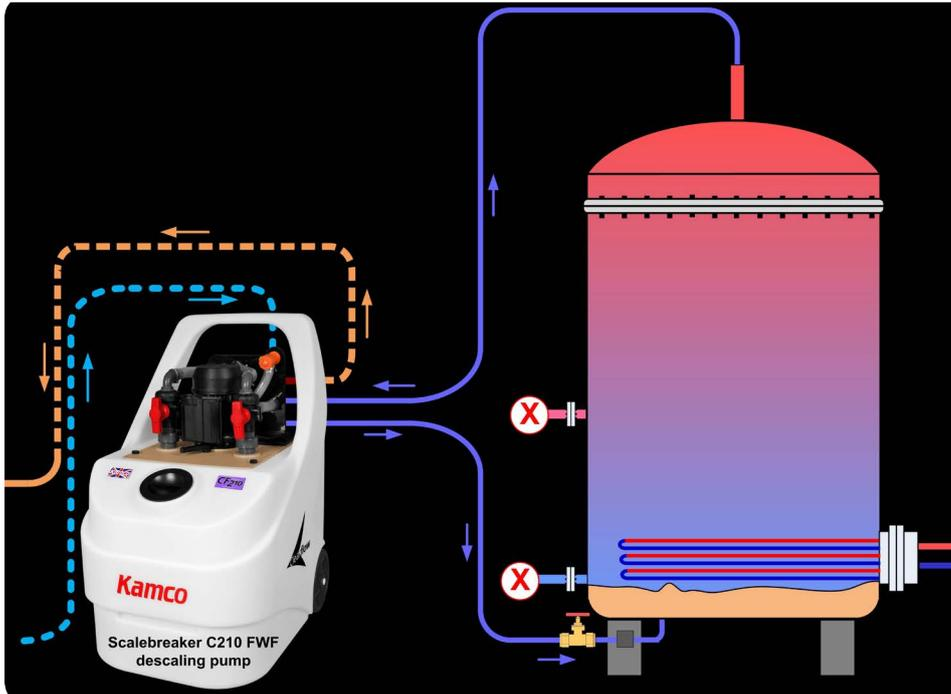
4. If there is a drain valve on calorifier, use this as pump connection point, in preference to the water feed inlet. Check that valve is clear and will pass water through at a reasonable rate. If necessary clear a passage through any blockage - there may be several inches of scale accumulation on the base of a calorifier.
